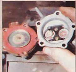
Mark the pump body halves before undoing the screws. In some pumps the valves are staked in position. In this event, clean out the valve locations with a scraper or fine file and stake in the new valves with a blunt dot punch.
