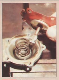
Rotate the diaphragm through 90° to remove it.
