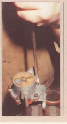
The top cap is part of the fuel chamber, hence the seal. There is also a neoprene seal between the cap and body. Check the pump for leaks when the system's
