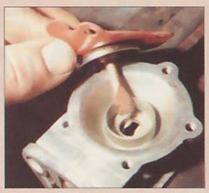
The diaphragm's centre pin fits bayonet-fashion into the slot in the link. In practice, ensuring the tab is turned by 90° does the trick. The diaphragm spring should be in place at this point, unless you're taking photographs...
