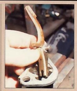
The lever, link and pin come out as a unit after the side retainers have been extracted with pliers. The anti-rattle spring can be seen in the lever chamber there is a locating pip for each end of the spring.
