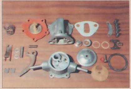
The entire assembly laid out with the contents of the kit. The above-mentioned retainers can be seen at the bottom left-hand corner. Make sure that the working area is clean.
