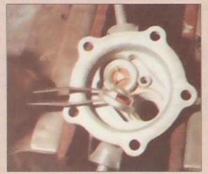
The AC pump is cast to accept the valves in the correct orientation, as you can see from the depth of the valve and of the hole which accepts it. Note the paper gasket in the valve location. The valves should be fitted with dissimilar faces showing.
