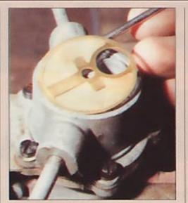
The brass filter screen is very delicate and should be removed carefully. Cellulose thinners will deal with gum deposits on all the metal parts.
