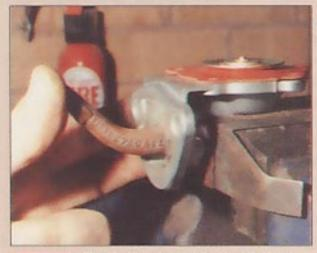
Push the lever in until the diaphragm is level with its mating face and hold it there whilst fitting the upper half of the pump body. With the screws fingertight, work the lever in and out to centre the diaphragm, then tighten the screws fully.
