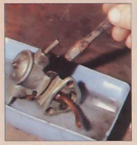
A paraffin bath will remove most of the accumulated filth from the pump before the strip down starts. Work the liquid into the lever chamber to get rid of the old oil.
