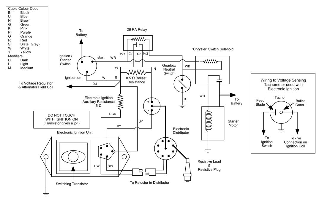
C.R.Foster 16/09/00 Wiring Diagram for BRISTOL 603 & 412, also 411 no 7680326 on Basic Ignition / Starter Switch Circuit Data from Bristol Cars SKN 6151
