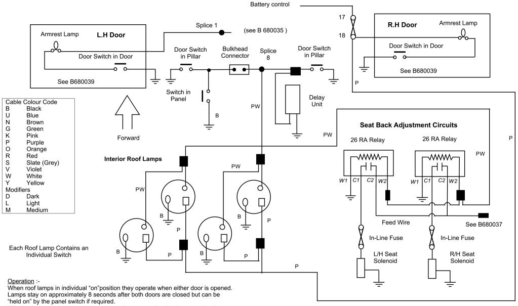
Warning lamps in door armrests operate when respective door is opened and are not affected by "delay" unit or panel switch.
